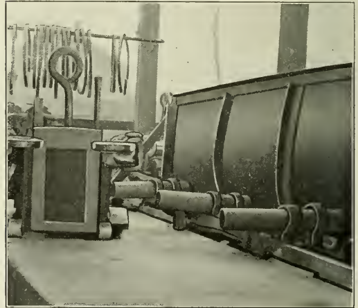
Fig. 5—Face Plate and Burners for Heating the Box Preparatory to Pouring the Brass.
